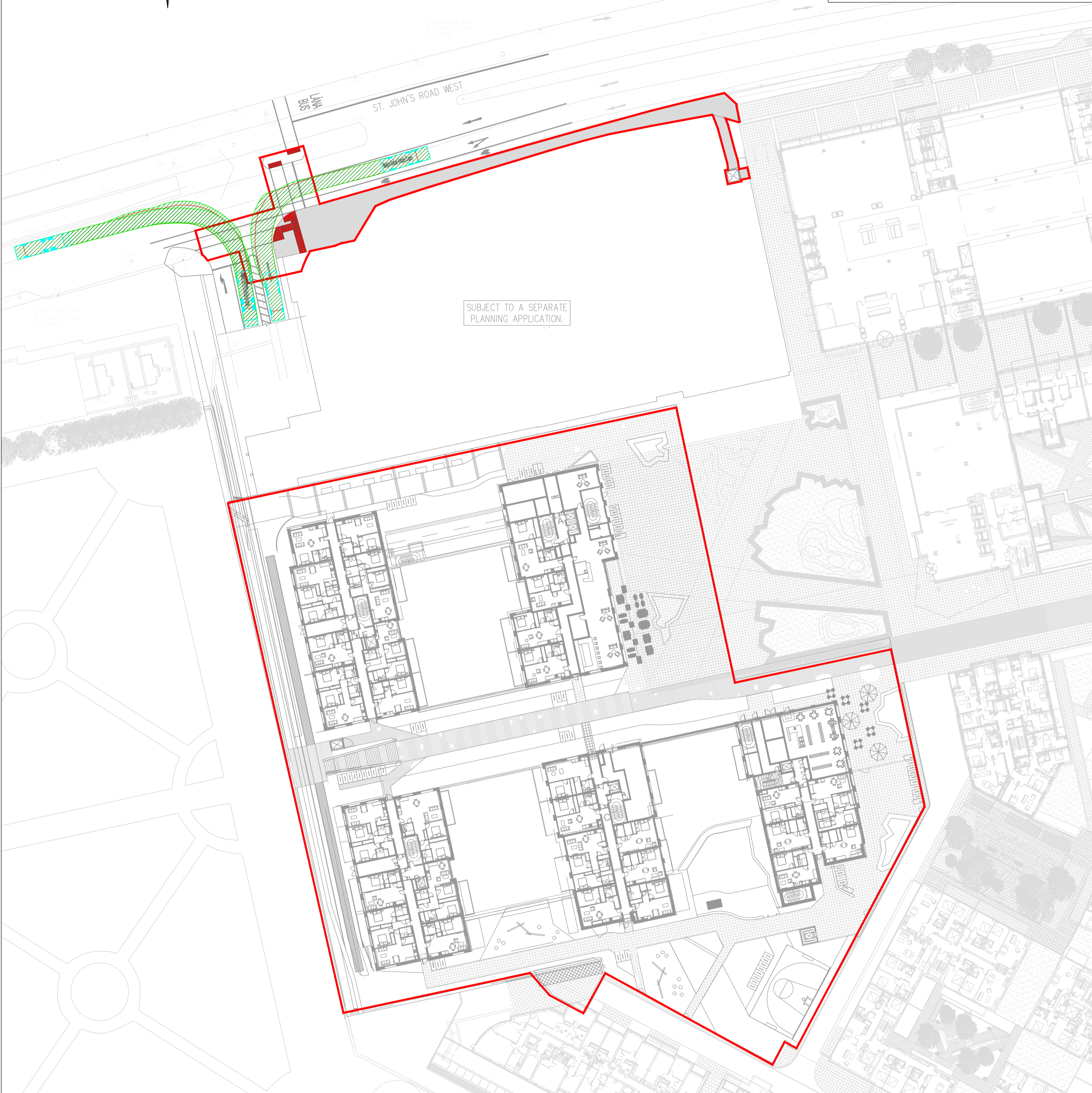
SWEPT PATH ANALYSIS-REFUSE VEHICLE, BASEMENT ACCESS. SCALE 1:500
